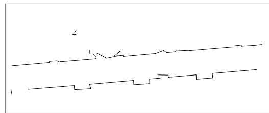
Fig. 9. Polyline map for the scan data depicted in Figure 8. This map contains 11 line sequences and 56 endpoints.
