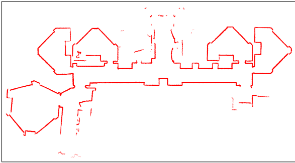
Fig. 6. Scan data and polyline map of the museum in Herakleion. The size of the environment is 38 times 18 m and the input data set contained 268,640 scan points. The resulting polyline map contains 62 polylines with 277 vertices.
