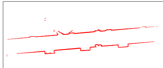
Fig. 8. Laser range data of a hallway at Stanford University. This data set contains 70,269 scan points.
